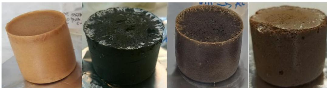
FIG. 1: Freestanding porous monoliths based on: VMT (a), AC (b), VMT-AC (c), AC-VMT (d)
