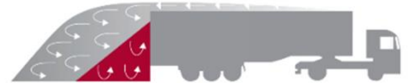
Turbulence zone with JOST SDR
