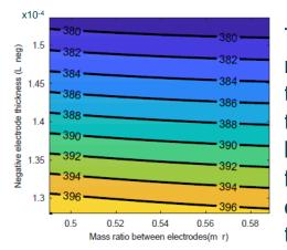
The impact of the negative electrode thickness is bigger than the mass ratio between electrodes for the power density response (in the analysed range)
