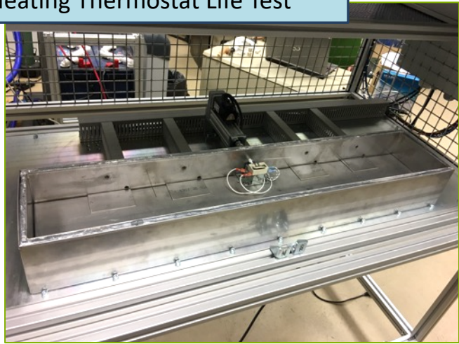
Radiant Heating Thermostat Life Test
